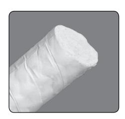
Yarn: braided in round cross sections from 100% pure, unsintered PTFEtapes. In order to achieve even better impermeability for fluids and gases wrapped with a layer of pure PTFE-tapes. Extremely pliable and durable, excellent chemical and thermal resistance. exceptionally low coeficient of friction. BAM approval.
